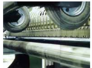
View of the application device with more than 100 adhesive application nozzles.
